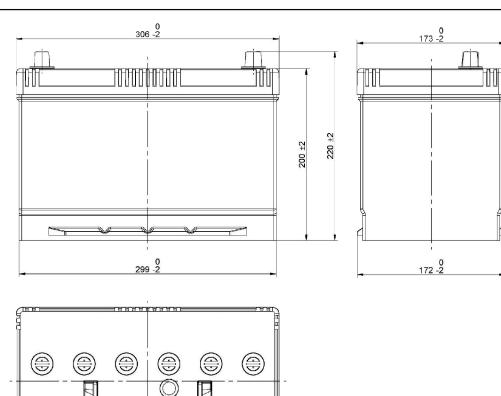
**PERFORMANCES CONTAINER** Type: D31 **BLACK** Voltage (V): 12 V Hold Down: Korean B1 20 h C20 (Ah): 90.0 H. D. Adapter: No Rc (min): 0 ΕN 680 Cranking (A): Vibration: V1 (35Hz/3g/2h) Endurance: E1 (180 cycles@25%) Charge: WET Technology: Vented/Flooded Grid: Ca/Ca WEIGHT AND STD. DIMENSIONS Battery Weight (kg): 22.32 Length (mm): 306 **PLUGS** Width (mm): 173 **BLACK** Type: 6 x M18 Height (mm): 222 **HANDLES** 1 x Integrated **BLACK** Type: **OTHERS** Degassing Tube: No
