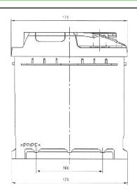
**PERFORMANCES** Voltage (V): 12 V 20 h C20 (Ah): 55.0 Rc (min): 0 ΕN Cranking (A): 460
